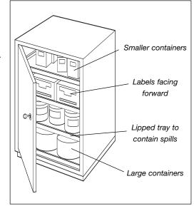
Caution: Never decant concentrate into an unlabelled container. Never re-use a concentrate container. Dispose of it safely or return it to the supplier. Don't store more than 50 litres of flammable liquid indoors. Use a flammables store.
